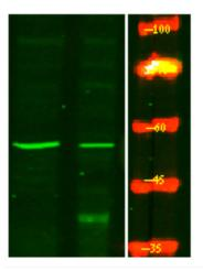
Western Blot analysis of Hela treated or untreated by LPS lysis, using primary antibody at 1:1000 dilution. Secondary antibody(catalog#:RS23920) was diluted at 1:10000
